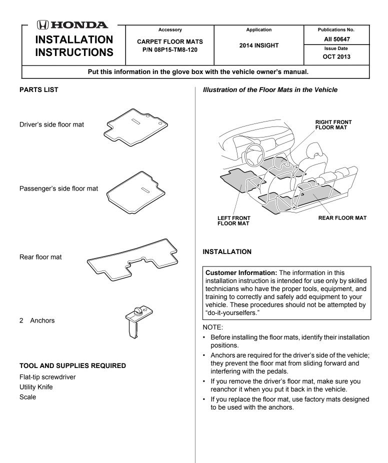
1. Install the driver's side floor mat over the anchors as shown.
